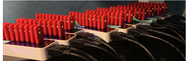
Figure 1: Our cluster of 100 low-cost hardware security modules (SoloKeys [72]) on which we evaluate SafetyPin.
